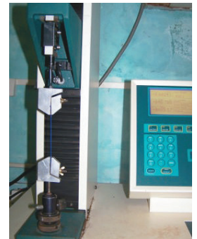
Fig. 1:Measurement of Tensile Strength of Specimens.
